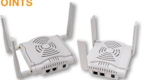
802.11n enables the use of wireless as a primary connection with speed and reliability comparable to a wired LAN. 802.11n increases performance through techniques such as channel bonding, block acknowledgement, and Multiple In Multiple Out (MIMO). In addition, advanced antenna technology also increases range and reliability.
