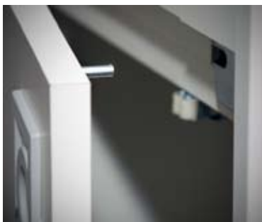
Safety features include automatically shutting off the shredder when the door is open.
