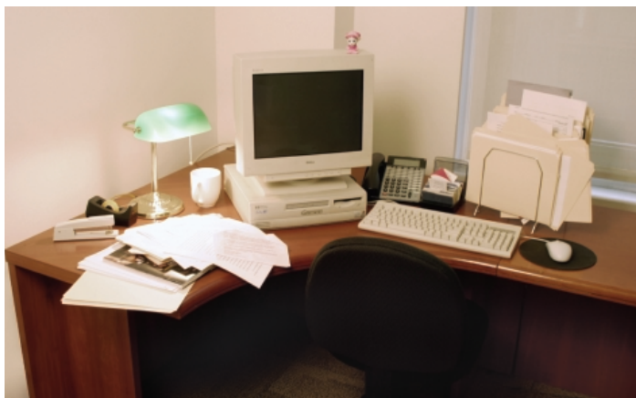
A poorly set-up workstation forces the user to twist in her seat and risk repetitive stress injury to the neck, back and shoulders. Here the monitor is misaligned with the keyboard and document surface, and the desktop is cluttered with the CPU, monitor, keyboard and mouse.
