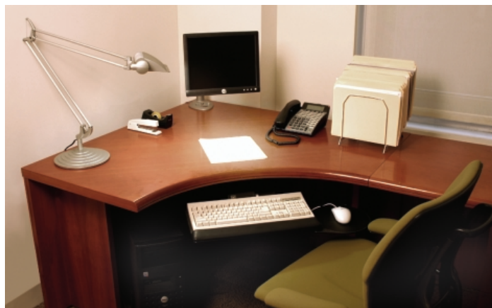
Use of a flat panel display supported by a monitor arm and a properly aligned, negative tilt keyboard tray will maximize the likelihood that the user maintains neutral postures throughout the day. The neck, back and shoulders align, and the workspace is clear of clutter with the CPU mounted under the desk and the monitor, keyboard and mouse off the work surface.
