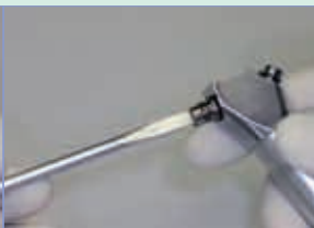
Using a screwdriver, unscrew existing syringe nozzle or converter
