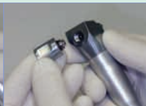
Screw the ProTip Converter on to the syringe body
